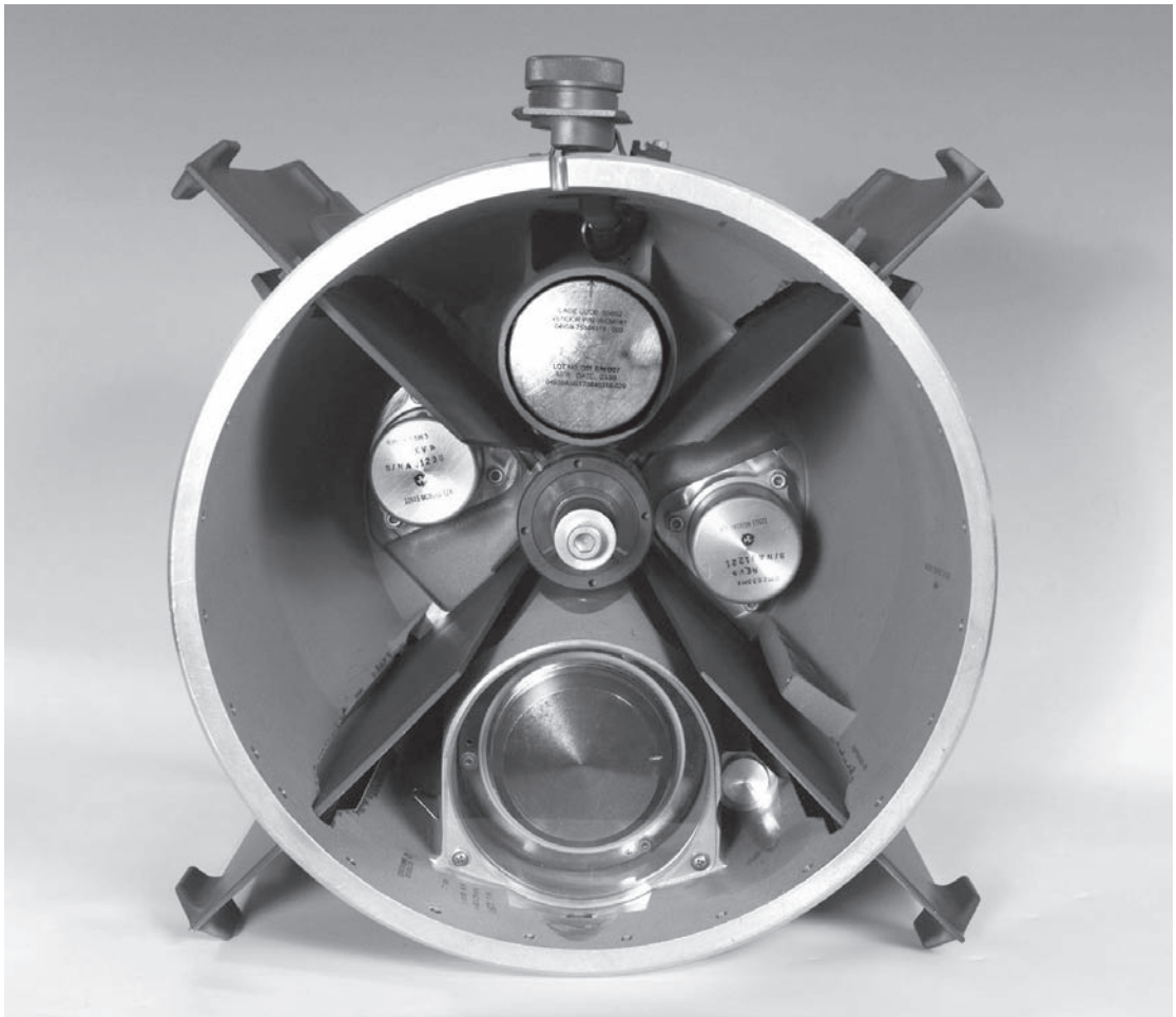
Figure 2. Microelectromechanical system inertial measurement unit. (From BAE Systems, Farnborough, Hampshire, United Kingdom.)
