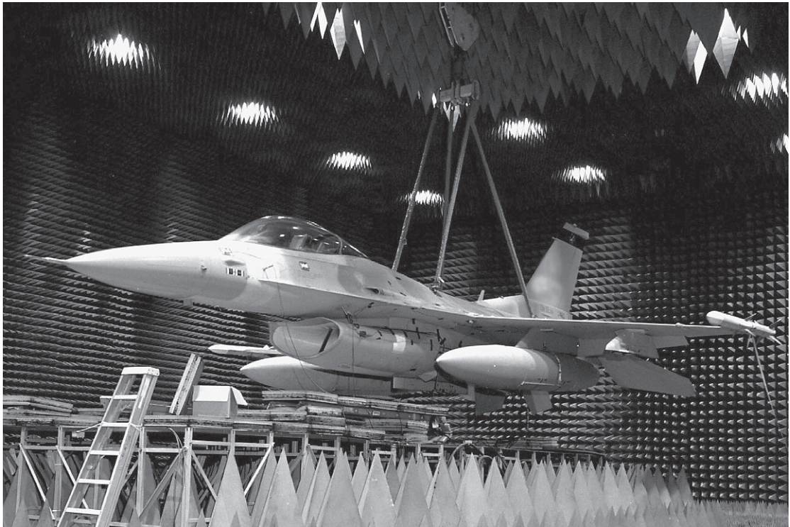
An F-16 suspended inside an anechoic chamber, which allows scientists to evaluate the aircraft's ability to guard against high-power microwaves
