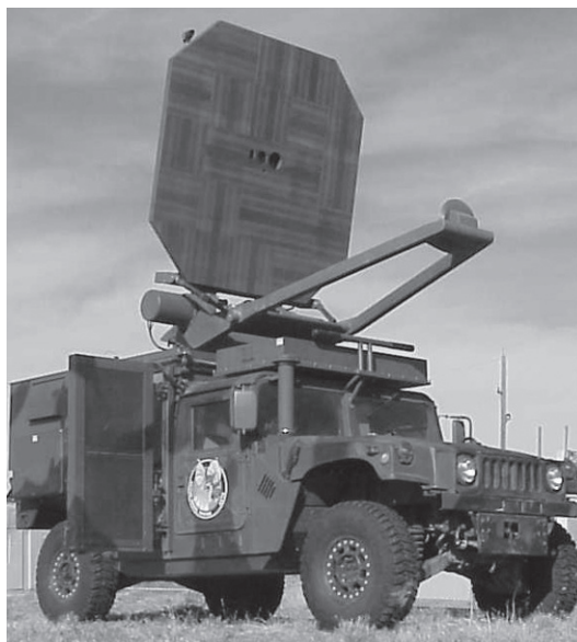
A military vehicle modified to carry active-denial technology, which uses a millimeter wave beam of energy to create an intense heating sensation that causes targeted individuals to repel or retreat
