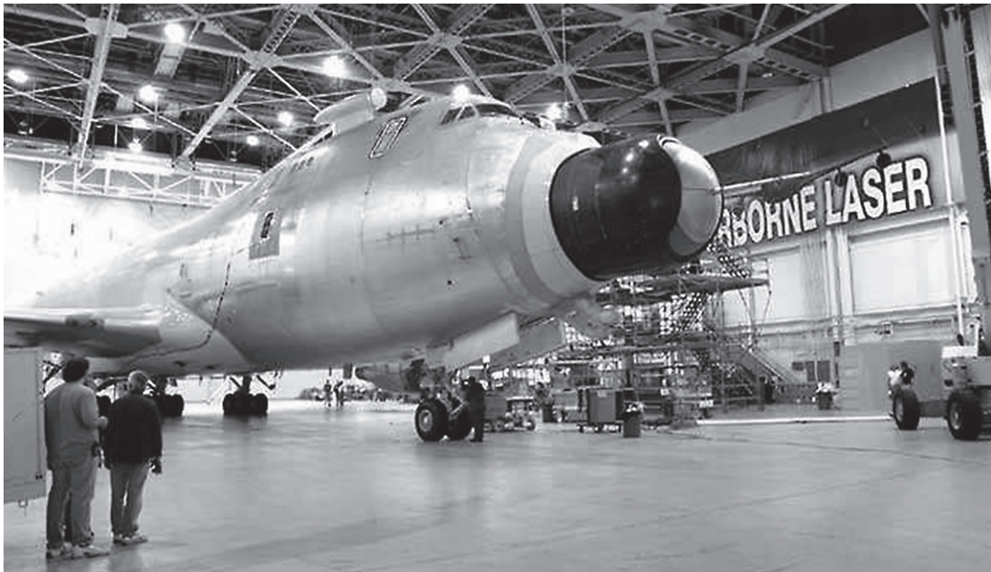
The airborne laser: a uniquely modified 747-400 freighter designed to shoot down ballistic missiles during their boost phase
