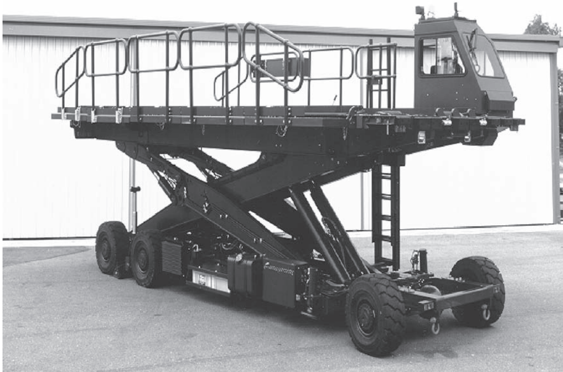
Figure 1. Next-generation small loader. (From Static Engineering Pty, Ltd., Adelaide, Australia.)
